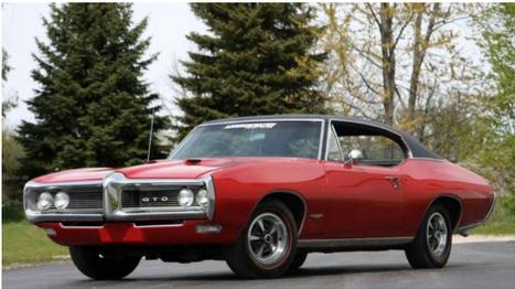
When the redesigned 1968 GTO hit the streets, it took Pontiac style to a new level with a pioneering monochromatic look unlike anything else in the market. Specifically, the front bumper was made from a malleable "Endura" polyurethane foam molded over a steel core, which became a GTO exclusive until 1970 (although Pontiac used it sparingly on select 1969 models). Starting in Decem-
