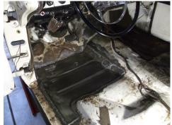
The panel is now welded all the way around. I've applied a rust reformer to the bare metal and any residual rust and then sealed and applied undercoat to the underside (a real treat that is).
