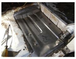
Next, the new panel is in place and body mount bolts are installed.
