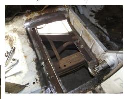
The back foot well floor pan repair followed the same procedures and this is what that job looked like. Here the rusty, perforated panel has been removed.
