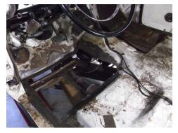
Next, I used a six-inch wire brush wheel (also Harbor Freight) in my large die grinder to thoroughly clean and de-rust the edges where I would soon be welding.
